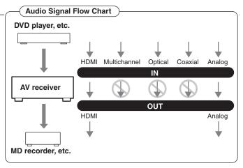
If signals are present at more than one input, the inputs will be selected automatically in the following order of priority: HDMI, digital, analog (including multichannel). You can specify which audio inputs the AV receiver checks for the presence of a signal in the "Automatic Audio Input Selection Setup" on page 49.
